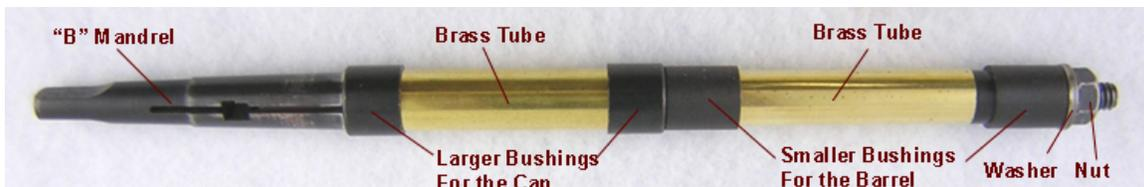
1. Assemble the blanks on the mandrel with the right bushings in the right place. The right bushing can be found by comparing the diameter of the bushing to the piece of hardware that will be placed in that place. For instance, the bushing that is the same size as the clip will fit on the end of the blank that will eventually become the top of the cap.
