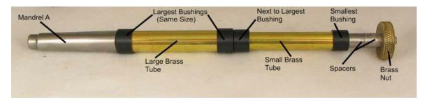
1. Assemble the blanks on the mandrel with the right bushings in the right place. The right bushing can be found by comparing the diameter of the bushing to the piece of hardware that will be placed in that place. For instance, the bushing that is the same size as the clip will fit on the end of the blank that will eventually become the top of the cap.
