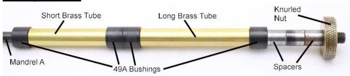
1. Assemble the blanks on the mandrel using the 49-A bushings. With these bushings it is not necessary to be particular with the order they go on the mandrel. They are all identical. Use a spacer take up the extra mandrel space.
