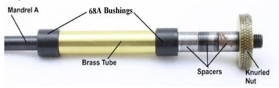
1. Assemble the blanks on the mandrel using the 68A bushings.
