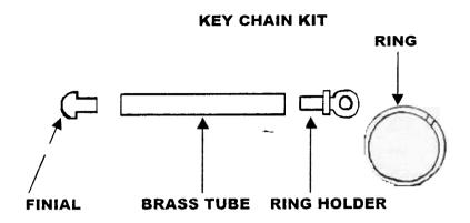
THE KEY CHAIN TUBE IS IDENTICAL TO THE TWIST PEN TUBE. THE SAME DRILL (7MM-LETTER J) AND MANDREL USED FOR THE TWIST PENS CAN BE USED HERE.
